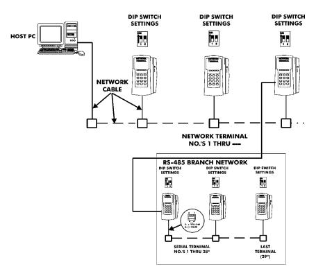
Note that the serial connections for the RS-485 branch network are the same as for the RS-485 wiring described previously.
