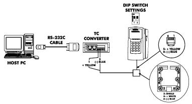
Note that when there is only one RS-485 terminal in the system, DIP Switch 1 must be in the ON position to enable the termination resistor.
