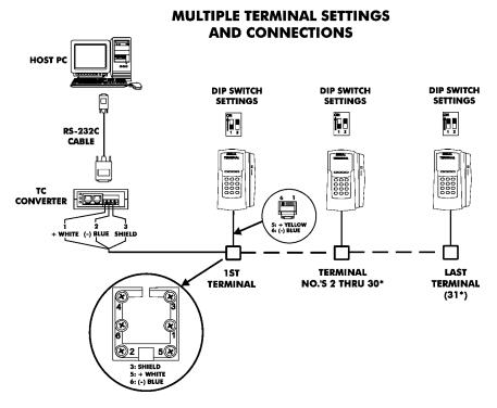
\* The maximum number of terminals is dependent upon the distance and the quality of cabling used. It is recommended that Belden Low Voltage Computer Cable, P/N 9841 or equivalent be used for this application.
